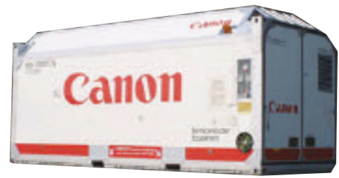
With double-layer air suspension to protect exposure devices from vibration, the ride in Canon's special shipping trailer is purported to be quite comfortable.
