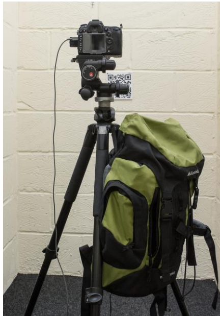
Figure 4 Hanging something heavy on the tripod can increase stability.
