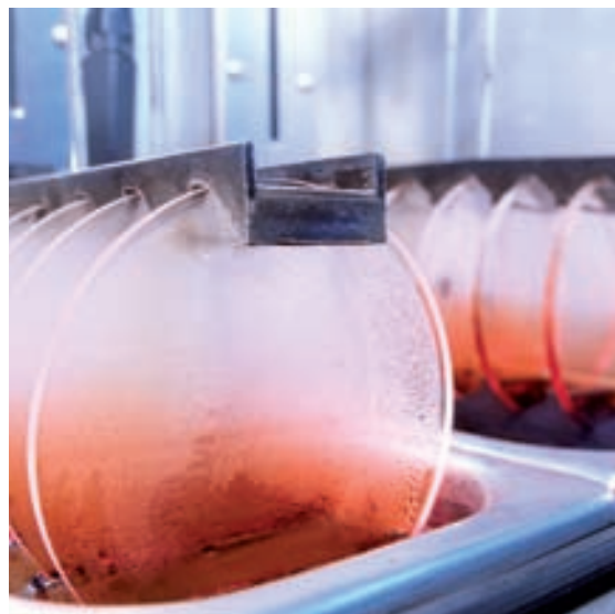
Amplitude-controlled immersion baths – this is how graduated filters are made
