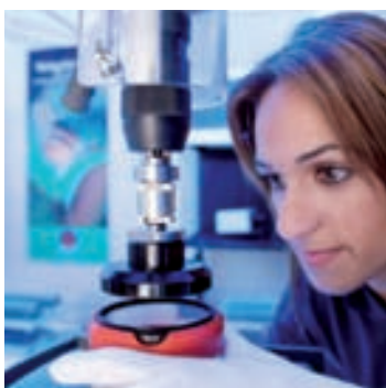
Filter assembly is performed carefully using torque-controlled equipment
