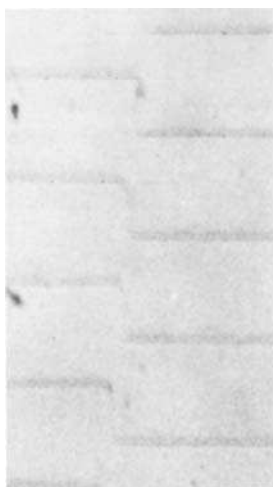
Fig. 1 Fringe pattern of a 154 nm thick \text{TiO}_2 film on glass. Multiple beam interferometry, \lambda=546 nm.
